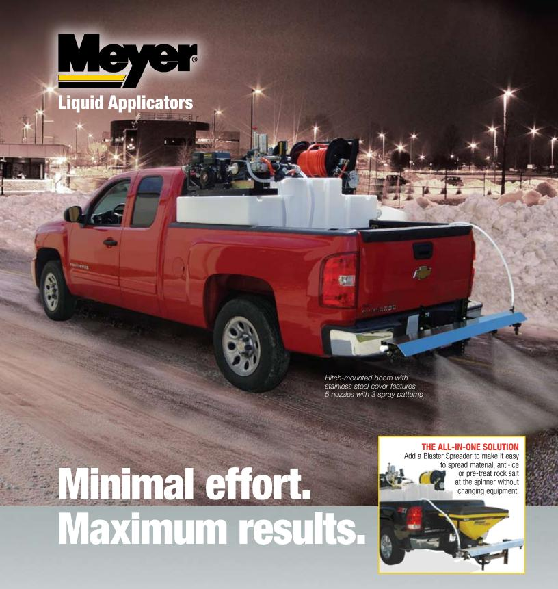
**Meyer® Anti-Icers**, with unique space saving design, are perfect for pre-treating areas that need to remain open during winter snow storms. When applied prior to the storm, the brine mixture will not allow snow or ice to bond to the pavement. Meyer anti-icers help contractors or municipalities become more efficient when the storm arrives by using less material and manpower to clear the area. And Meyer's space saving design allows users to carry other equipment.
